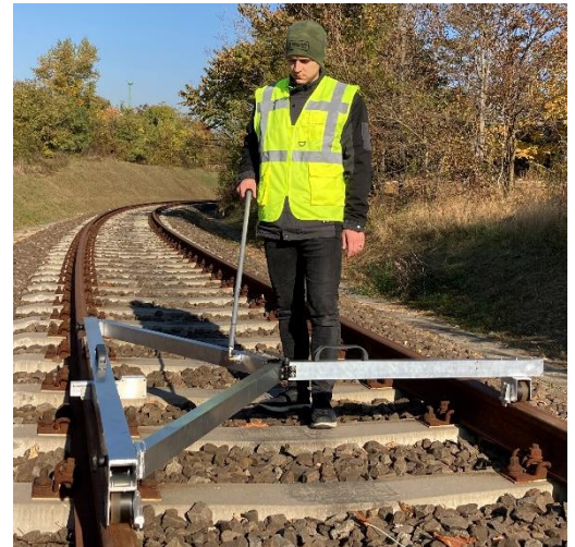
Figure 1.: The CHORD-2 device in track
